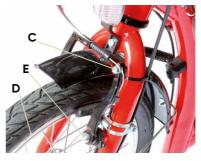
do this, loosen the clamping screw  $(\mathbf{C})$ , press the brake blocks together by hand, pull the Bowden cable taut and then re-tighten the clamping screw. If the brake blocks are not accurately aligned with the rim edge  $(\mathbf{D})$ , you must readjust them accordingly. In order to change the alignment of the brake blocks, loosen the screws  $(\mathbf{E})$ . Leave this work to your specialist dealer in case of any uncertainty.
