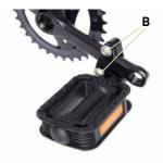
the maximum flexion of the knee is to be achieved. This adjustment is to be undertaken in interaction with the saddle height. In order to adjust the continuously adjustable cable shortener, loosen the screws (**B**) and bring them into the required position.
